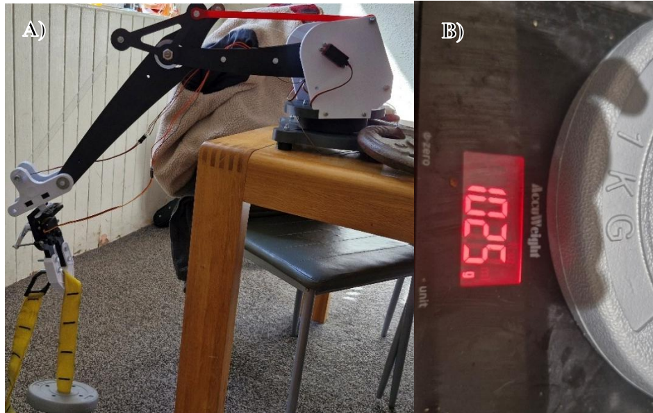
Figure 29 – A) Robotic arm holding 1Kg at full extension, B) Calibrated mass
