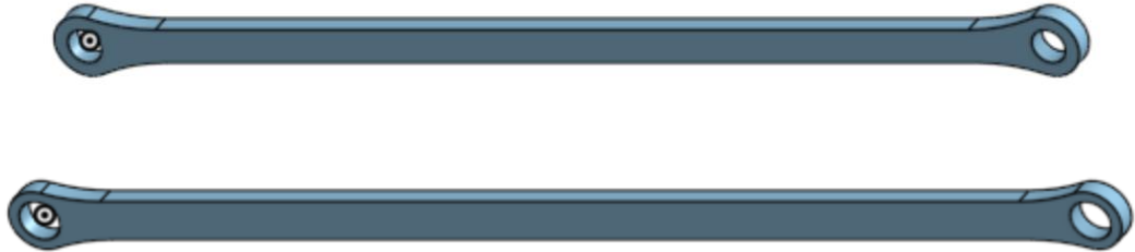
Figure 20 - Arm 2 (support-pivot) & arm 3 (joiner arm-slider/pivot-gripper head)
